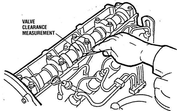
If the valves clearances are not within the standard values, use the following procedure to adjust the valves.
