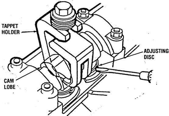
**EXAMPLE (Intake Valve):** The thickness of the disc removed plus the clearance measured minus the standard clearance will give the thickness of the new adjusting disc.
