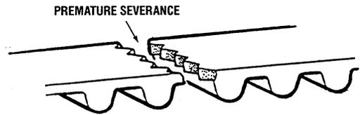
2. Check the teeth for damage, cracks, peeling and hardening, and check for any missing teeth.
