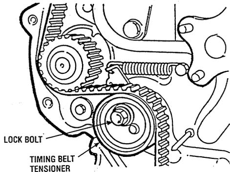
4. Turn the crankshaft twice in the direction of normal engine rotation (clockwise) to equalize tension on the timing belt.
