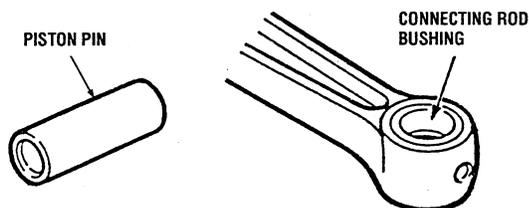
2. To replace the connecting rod bushing, use a press and a suitable pipe (diameter = 27 – 27.5 mm (1.06 – 1.88 in)).
