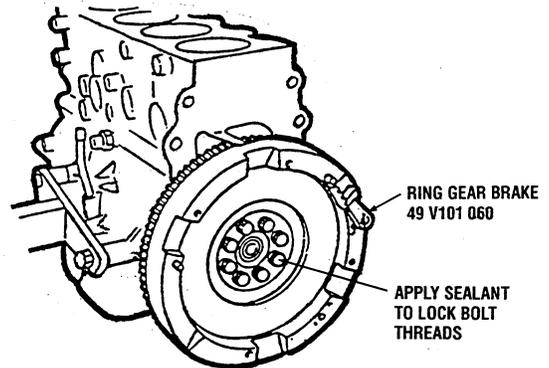
3. Install the damper plate onto the flywheel.
