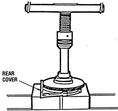
3. Install the rear cover assembly over the gasket.
