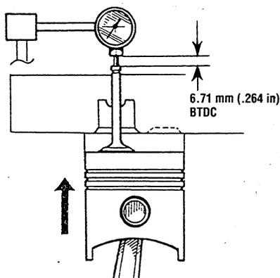
2. Turn the crankshaft until the indicator shows the valve drop to be at .264 inch. This is 30° BTDC.
