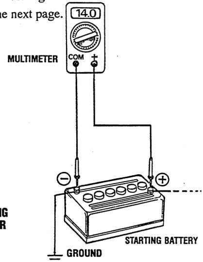
TESTING THE STARTING BATTERY-ALTERNATOR (ENGINE RUNNING)
