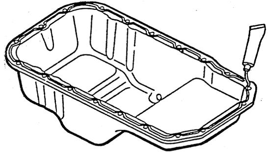
2. If a gasket is used, apply *PERMATEX* sealant (or equivalent) to the areas indicated by the arrows in the illustration after first cleaning the surface where the oil pan meets the cylinder block.
