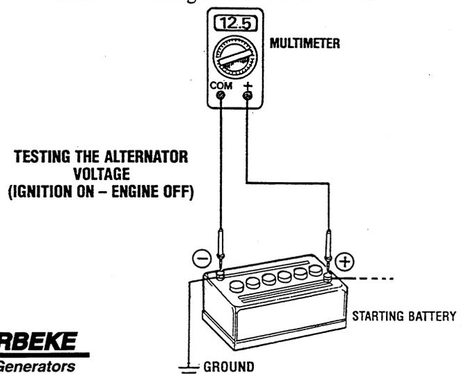
TESTING THE ALTERNATOR VOLTAGE (IGNITION ON - ENGINE OFF)
