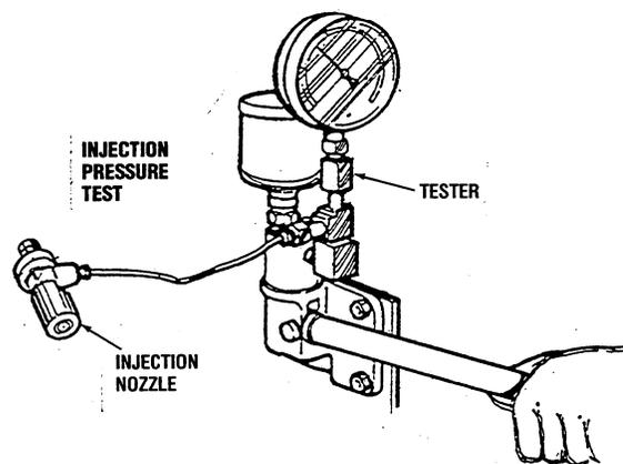
7. If the injection starting pressure of the nozzle is not within the limit, loosen the cap nut on the nozzle holder, insert a flat screwdriver through the bolt hole of the cap nut, then turn the pressure adjusting screw to set the injection starting pressure to 200 kg/cm<sup>2</sup> (2.844 lb/in<sup>2</sup>). Then, gradually decrease the pressure until the injection starting pressure is 135 kg/cm<sup>2</sup> (1920 lb/in<sup>2</sup>).
