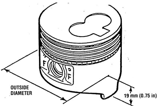
3. Inspect the piston rings for damage, abnormal wear or breakage. Replace if necessary.
