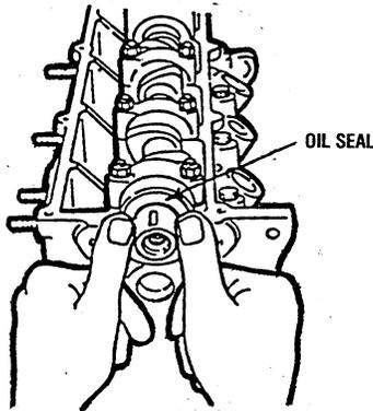
5. Tighten the camshaft cap nuts to the specified torque. See *Cylinder Head, 5.*, under *ENGINE INSPECTION AND REPAIR* for measurement of the oil clearance.
