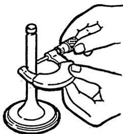
**CAUTION:** After the valve guide is replaced, recheck the gap between the valve and the valve guide.
