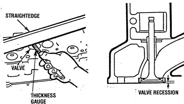
2. Check the surface which contacts the valve face for roughness or damage. If necessary, use a valve seat cutter or valve seat grinder to repair to the specified shape.
