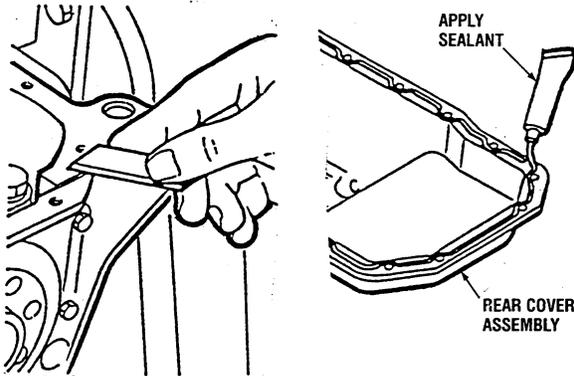
**CAUTION:** Before application, remove any dirt or grease from the contact surfaces with a rag. Apply sealant only to the cylinder block or the oil pan, not to both. After the sealant is applied, the pan must be secured within 30 minutes.
