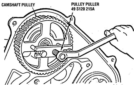
3. Remove the timing belt pulley.
