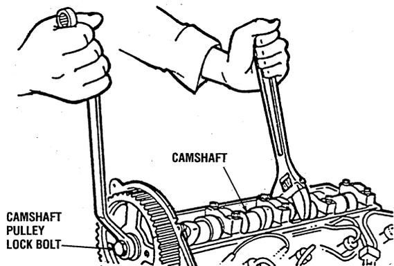
**CAUTION:** Do not damage the edge of the cylinder head with the wrench. If it is damaged, engine oil may leak.
