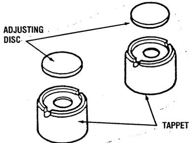
**NOTE:** The number marked on the disc indicates its thickness. Example: 3825 means 3.825 mm (0.1056 in). Adjusting discs are available in 25 different thicknesses between 3.40 and 4.60 mm (0.1339 - 0.1811 in) at variations of 0.050 mm (0.002 in).
