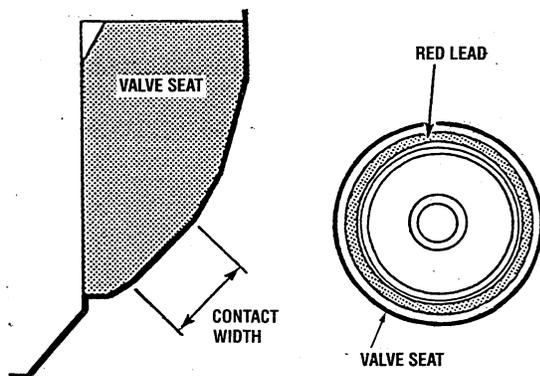
**NOTE:** When grinding the valve seat, use a 15°, 45° or 60° valve seat cutter or valve seat grinder to grind away the roughness and/or scars (to the minimum limit) of the seat surface, always checking the contact width and contact position while grinding.
