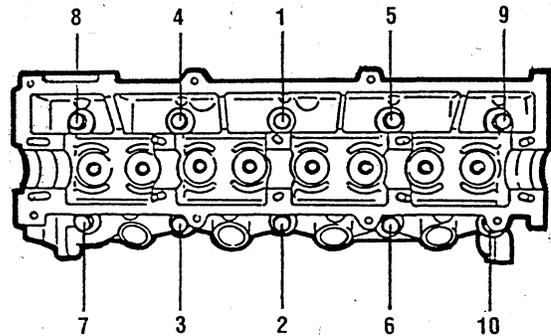
TIGHTENING THE CYLINDER HEAD BOLTS
