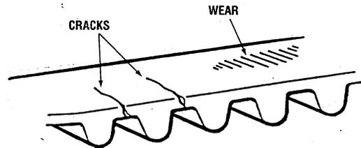
4. Check for wear or damage on only one side of the belt.
