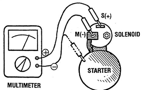
**NOTE:** Disconnect the wire from terminal M.
