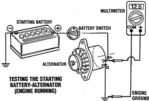
F. Start the engine again. Check the voltage between the alternator output and ground.
