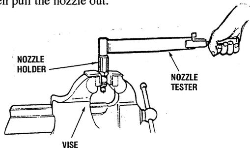
**NOTE:** The greatest possible care should be taken when handling the nozzles, as they are very precisely machined. The nozzle and the needle valve are matched pairs — do not mix their original combinations.
