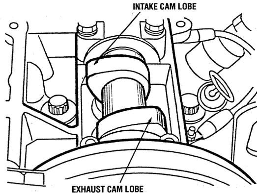
3. Measure the valve clearance of the #1 cylinder by using a thickness gauge.
