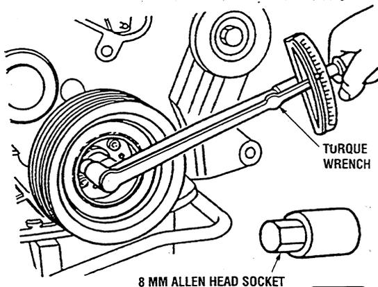
6. Recheck the timing mark positions between the three pulleys and the seal plate. Check the timing belt deflection with a pushing force of 10 kg (22 lb) at the point on the belt shown in the illustration.
