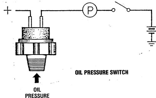
When the oil pressure drops to 5 – 10 psi (too low), this switch interrupts the circuit for the fuel run solenoid by opening, thereby shutting down the engine. This switch also activates an alarm that emits a pulsating signal when the oil pressure drops to 5 – 10 psi.
