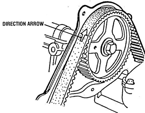
3. Loosen the timing belt tensioner lock bolt to allow the timing belt tensioner to bring pressure on the timing belt.
