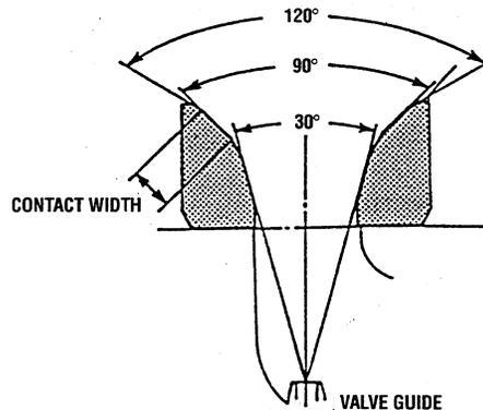
3. To seat the valve, apply a thin coating of engine oil mixed with a small amount of compound to the seat surface, then lightly tap while turning the valve.
