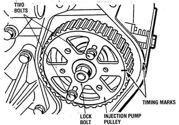
3. Using the pulley puller (49 S120 215A), separate the injection pump pulley from the injection pump shaft.
