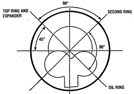
**CAUTION:** Apply a liberal coat of engine oil during installation. The rings must be mounted so the "R" or "RN" marks face upward.
