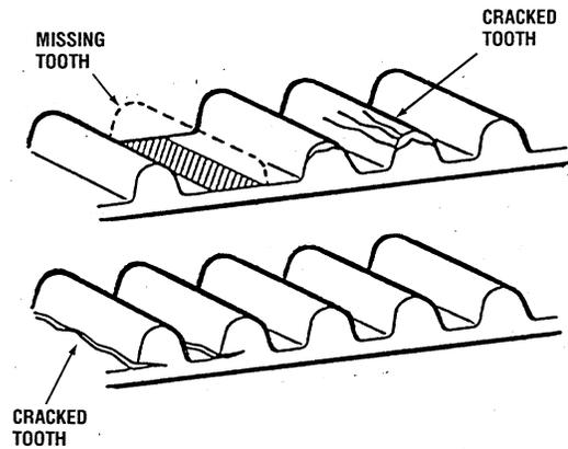
3. Check for noticeable wear or cracks on the belt face.
