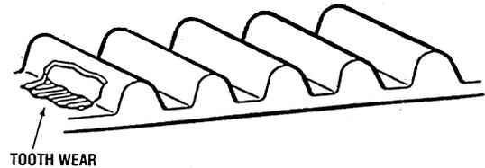
**CAUTION:** Never forcefully twist the timing belt, turn it inside out or bend it. Be careful not to allow oil, grease, or moisture on the belt.
