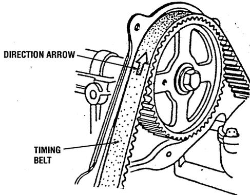
1. Loosen the timing belt tensioner lock bolt, push the timing belt tensioner left as far as it will go, then temporarily retighten the lock bolt.
