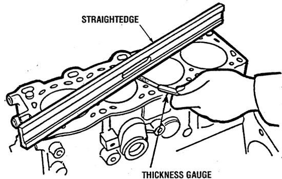
3. If the distortion exceeds the limit, replace the cylinder block.
